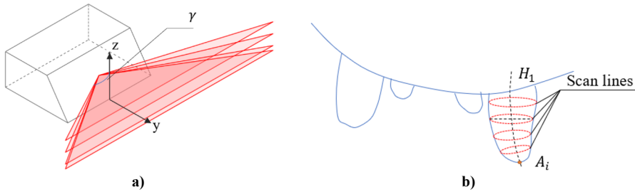
Fig. 4. Operation of the UPS: a – schematic representation UPS; b – detection objects.
