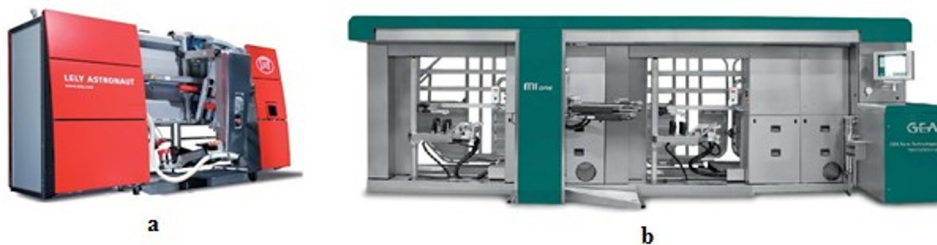
Fig. 2. Single and multi-box milking robot.
