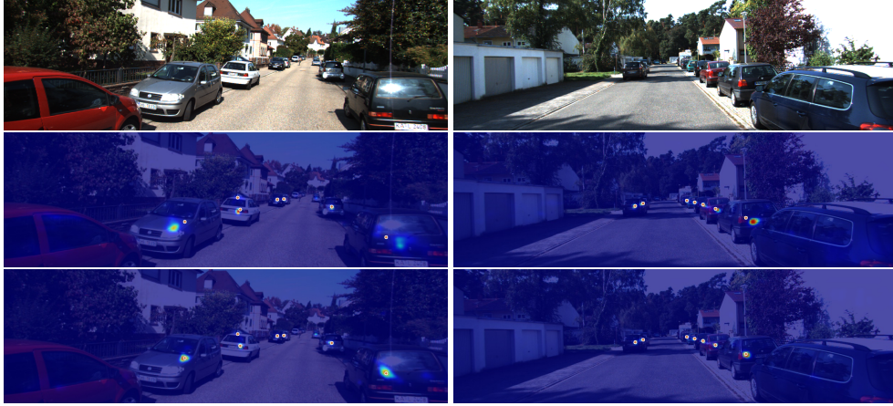
Figure 3.7: Qualitative comparison for the learned features of coarse center detection task on the KITTI-3D validation set. Top: the input image. Middle: the features of the coarse center detection branch supervised by the 2D center. Bottom: the features of the coarse center detection branch supervised by the projected 3D center. We use the white circle to highlight the ground truth projected 3D center for better comparison. Best viewed in color with zooming in.
