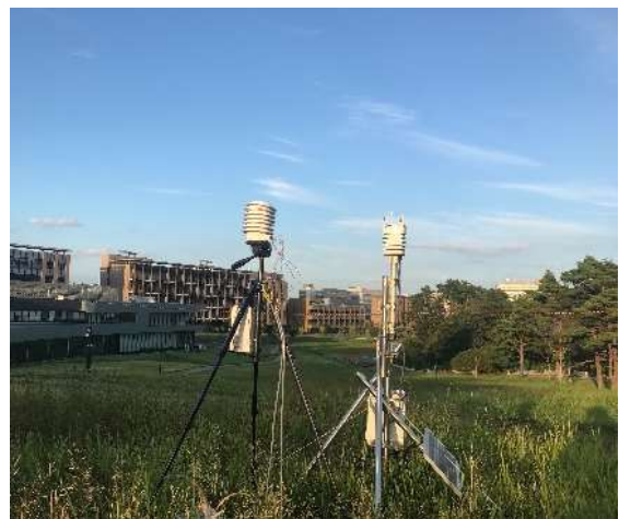
Photo 2 Test observation of air temperature and air humidity sensor with 3D-printed radiation shield. Left side is developed system and right side is WXT536 for validation.
