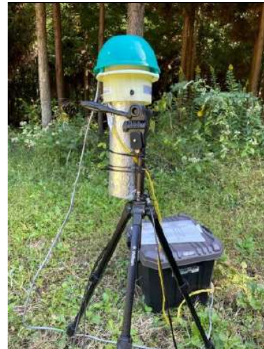
Photo 4 Test observation of air temperature and air humidity sensor with forced ventilation system.
