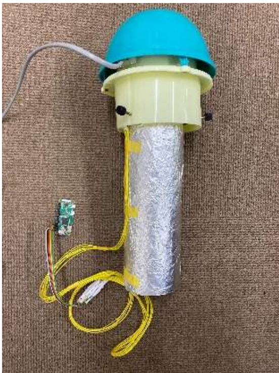
Photo 3 Forced ventilation system
