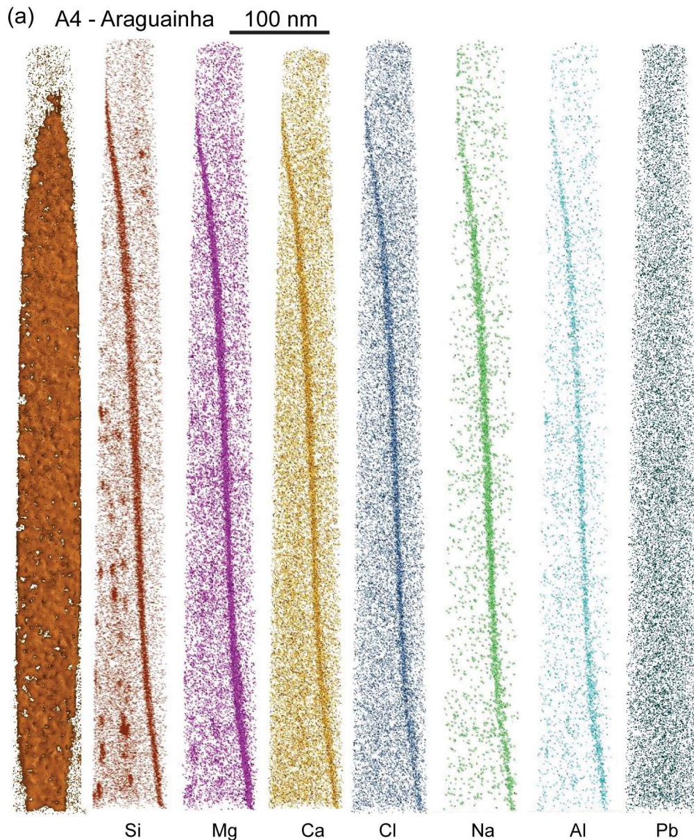
Figure 5.10: Specimen A4 from Araguainha showing grain boundary enriched in elements such as Si, Mg, Ca, Cl, Na, Al. The specimen also shows the presence of Si-Mg clusters distributed variably in different grains.
