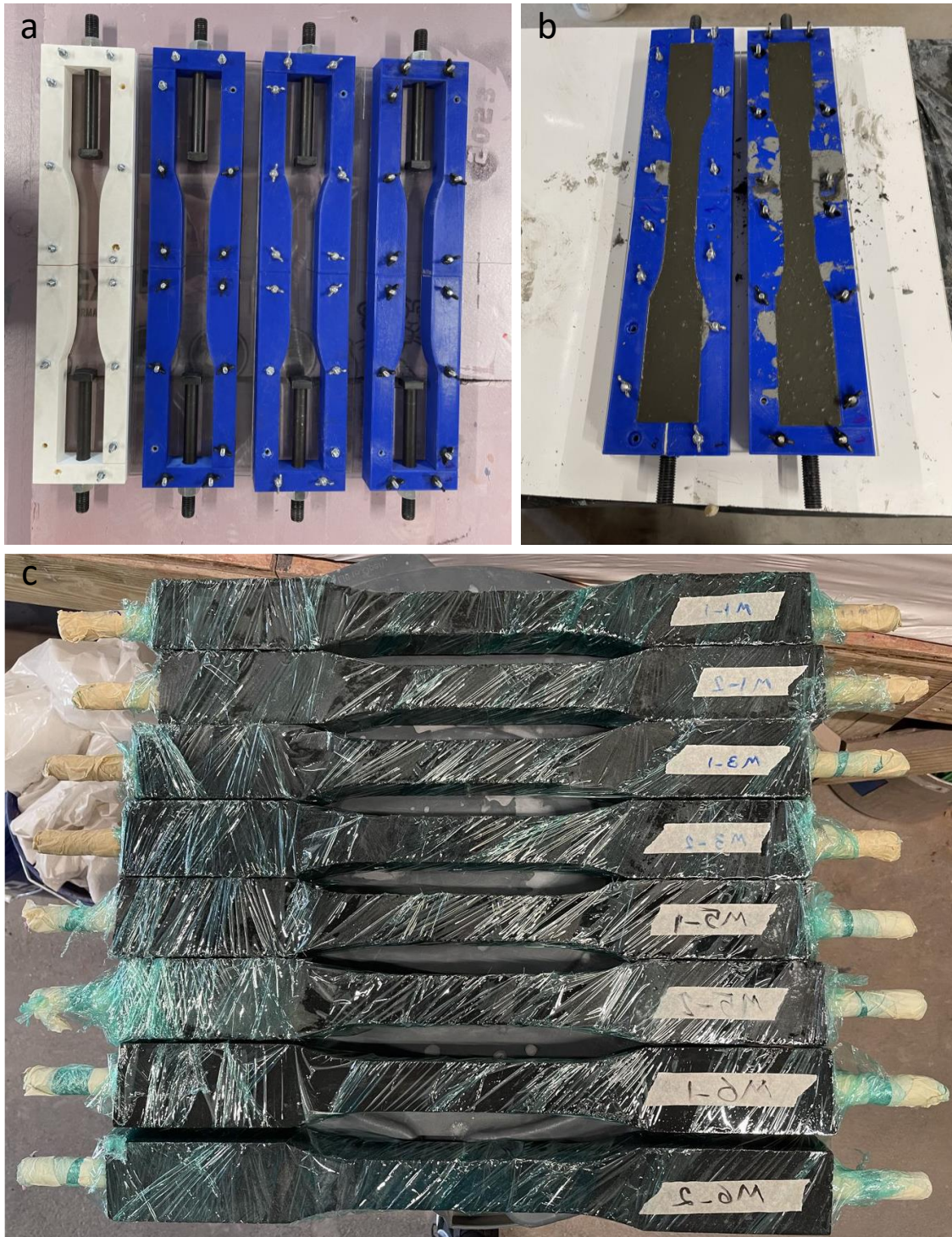
(a) the 3D printed mold for the dog-bone specimens, (b) casting of the dog-bone specimens, and (c) dog-bone specimens for tension test.
