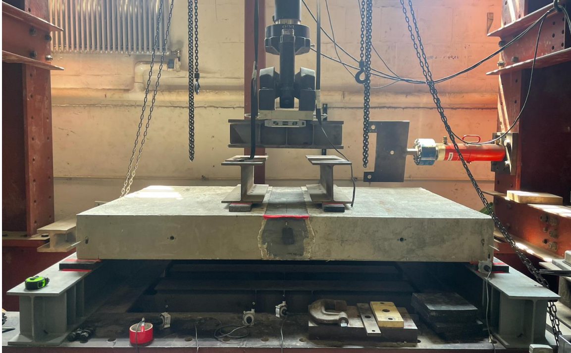
Figure 7.5: Finalized closure pour test setup
