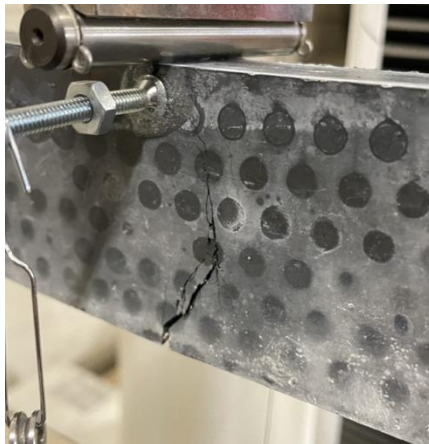
Figure 5.28: Crack in UHPC beams under flexure loading
