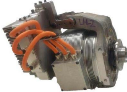
Figure 13: Air cooled in-wheel drive system developed within the FP7 programme EUNICE project (from [240]).
