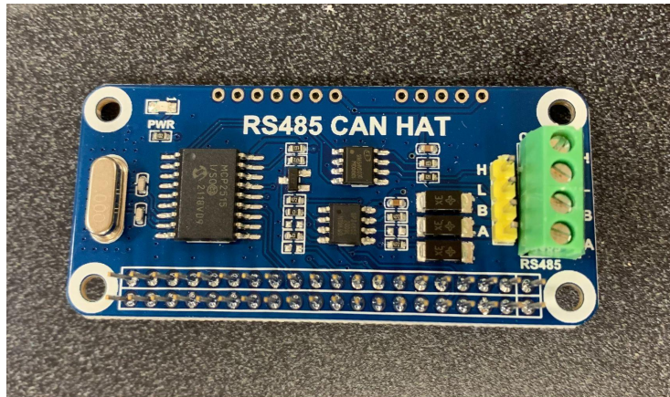
Figure A.3 An RS-485 CAN HAT provides serial communication between the DCM and the DER.
