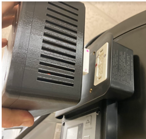
Figure B.3 Through holes on DCM aligning with brass nut inserts on the adapter module for correct orientation.
