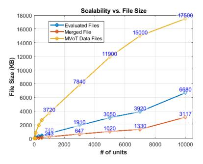
**Figure 3.6** The impact on the file size at the CDTA as the number of DTMCs increased from 1 to 10,000.
