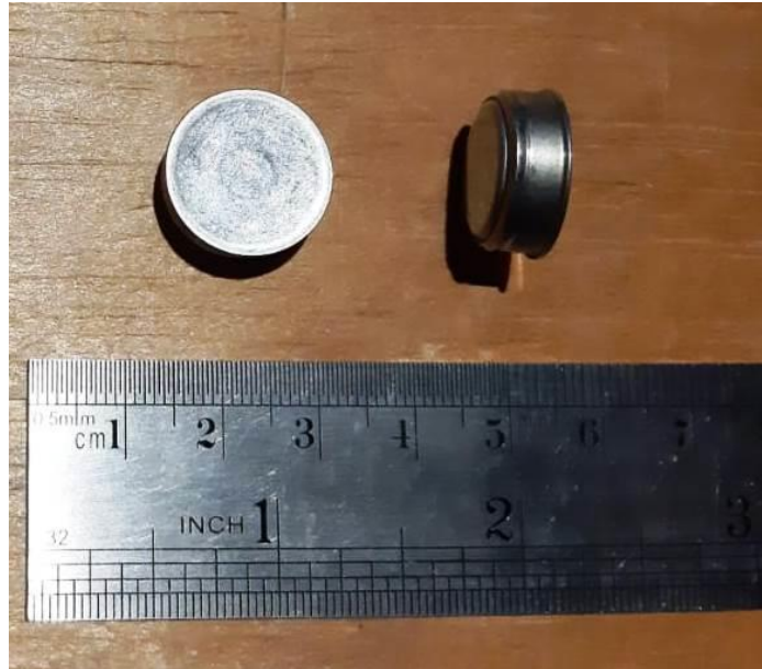
Figure B6. Stove use monitors (SUMS) are small devices that are placed on stoves to record surface temperature
