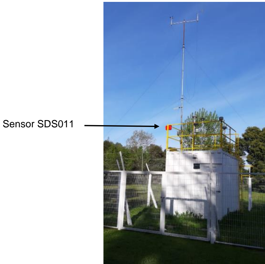
Figure B5. Comparison between our SDS11 PM2.5 sensor and the reference Air Quality Sensor
