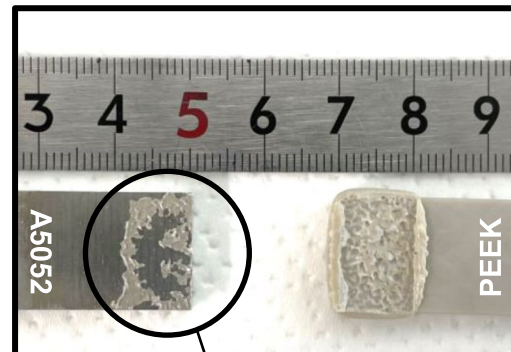
Interface delamination + Extensive PEEK cohesive breakdown
