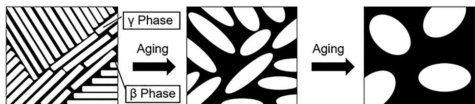
Fig. 13 Schematic of coarsening of microstructure in Sn–In solder during thermal aging
