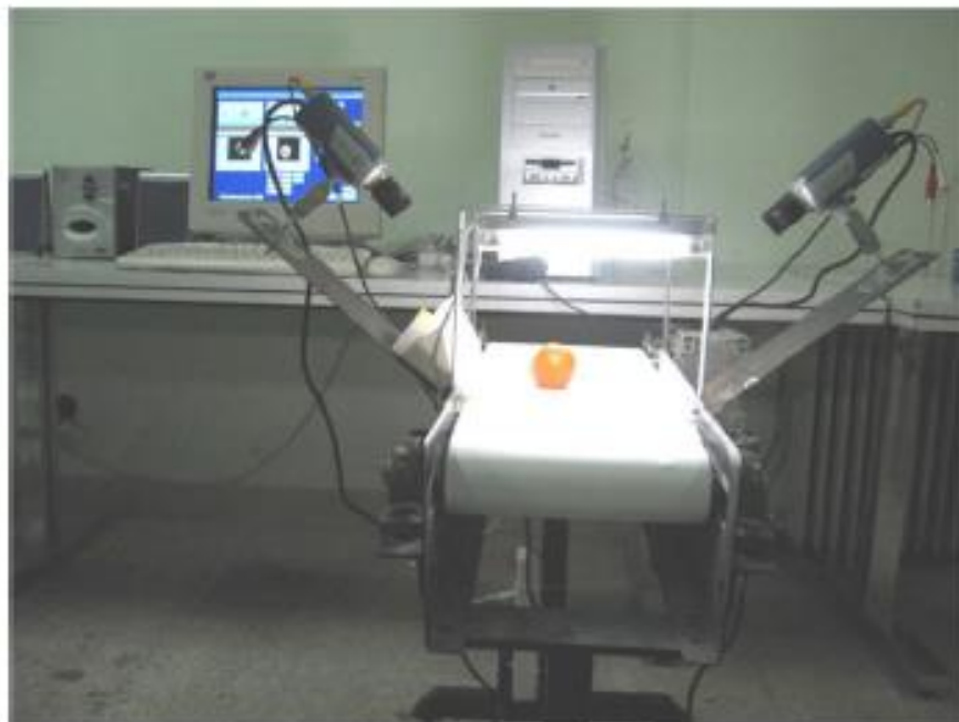
Figure 2.5: Estimate Mass and Volume of Citrus Fruits by Applying Image Processing
