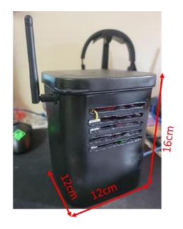
Figure 4. 2 Dimension of the enclosure
