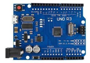
Figure 3.9 Arduino Uno R3 Microcontroller Board[34]
