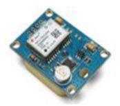
Figure 3. 12 GPS NEO-7M Module[38]
