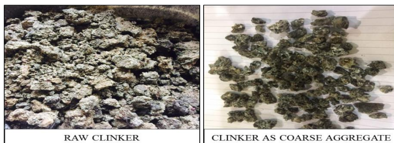
Figure 3. Palm oil clinker before and after processing
