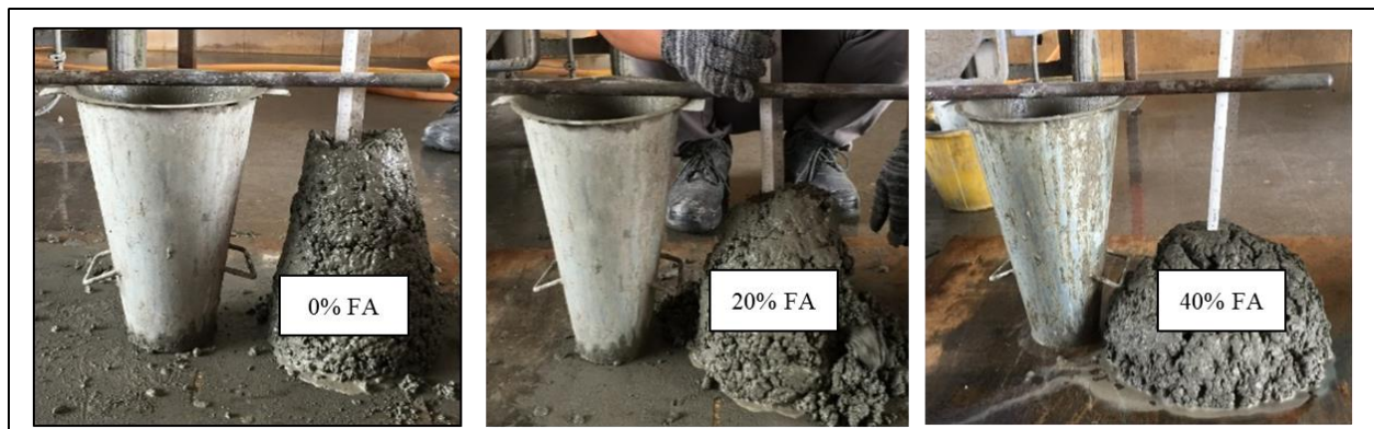
Figure 6. Effect fly ash on slump pattern
