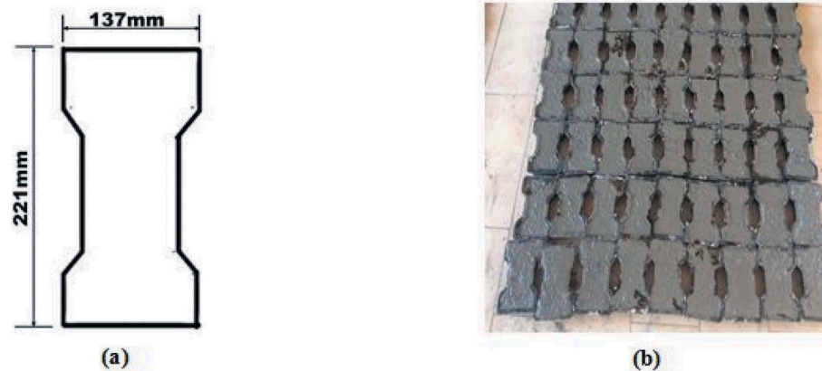
Figure 1. (a) Schematic of dog-bone mold (b) fresh mixture in mold.
