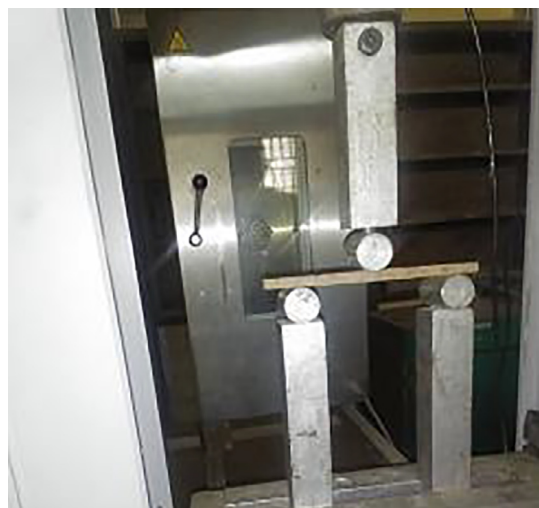
Fig. 4. Flexural test set up for the specimen.
