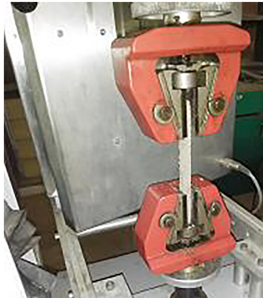
Fig. 3. Tensile test set up for the samples.
