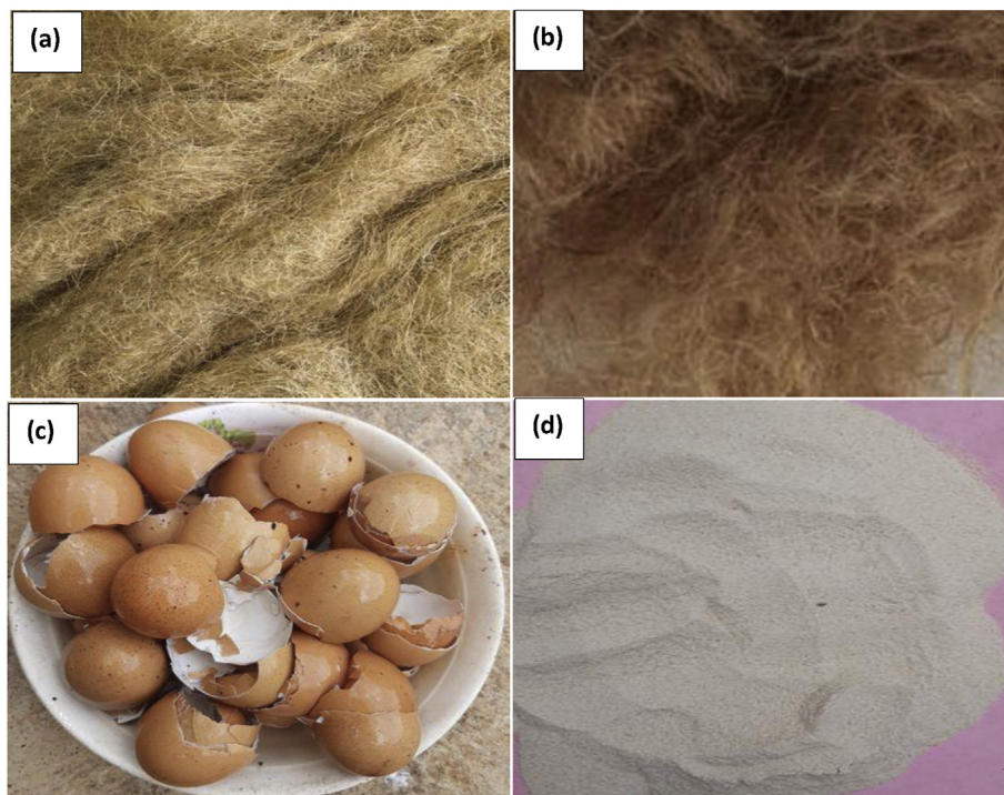
Figure 1. Showing (a) Untreated Jute fiber (b) Treated jute fiber (c) Eggshell and (d) Pulverized eggshell.
