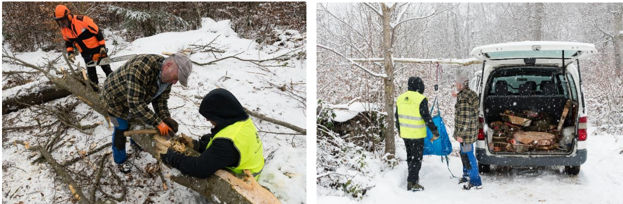
Figure 5: Scraping bark of a stem wood (left). Two members of the staff weigh a stem disk in the field. In the car, the already sampled stem disks are visible (right) (Speich 2021).
