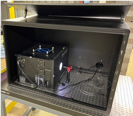
(a) Mobile test station for evaluating COTS VIS EBCs
