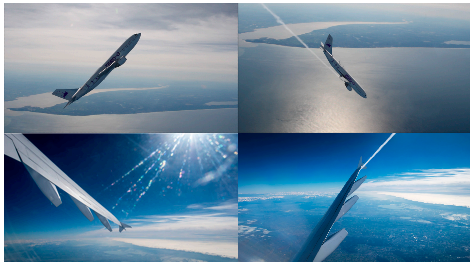
Figure 2. Induction and termination of the Keplerian free fall trajectory with the Airbus A310 ZERO-G. Left: Pull-up maneuver with an angle of approximately 50 degrees and an acceleration of around 1.8 g for 20 s. The engine thrust is then reduced to the minimum required to compensate for aerodynamic drag. The aircraft then follows a free fall trajectory of approximately 22 s, as well as between \pm 2.10^{-2} g in the z axis and between \pm 10^{-2} g in the x and y axes. Right: Pull-out maneuver of approximately 20 s and 1.8g for a return to normal level flight attitude (Pictures: Novespace/R. Sablotny).
