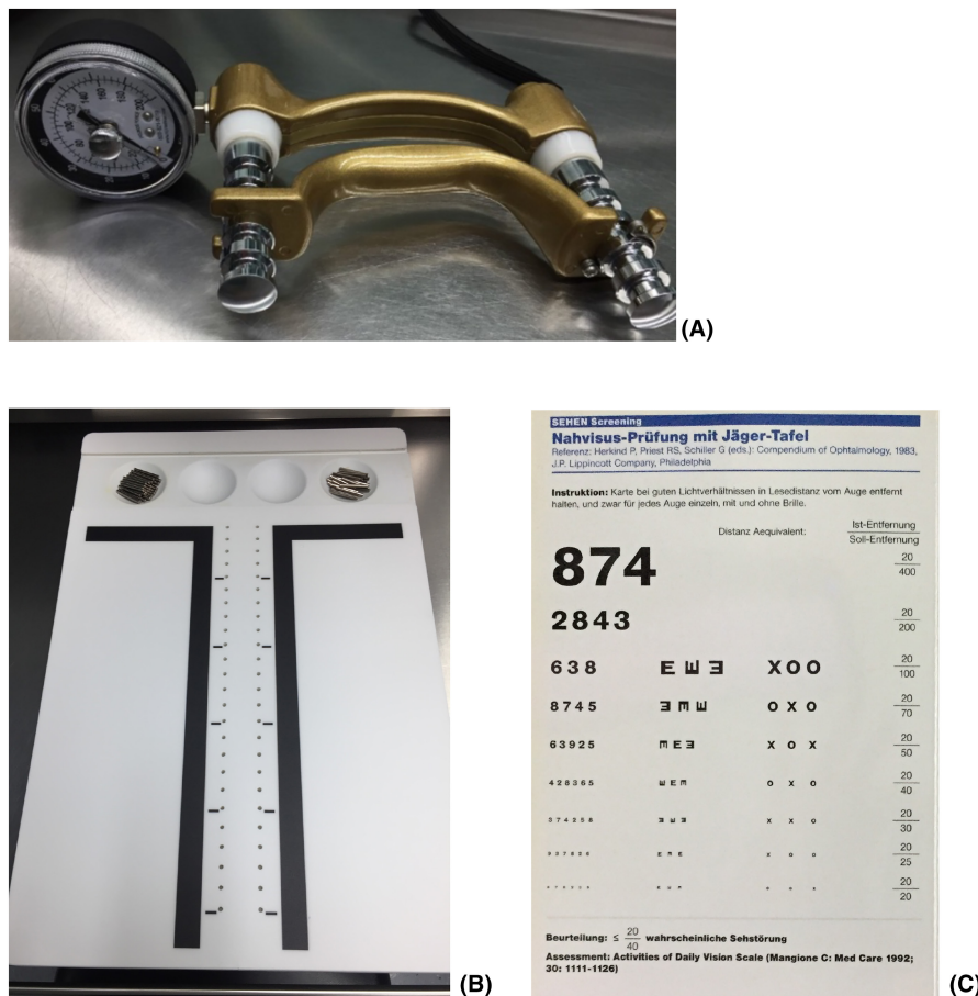
FIGURE 1 Overview of the measuring instruments to assess (A) handgrip strength (JAMAR®-Dynamometer), (B) manual dexterity (Purdue® Pegboard) and (C) visual acuity (Jaeger chart. 33 ).
