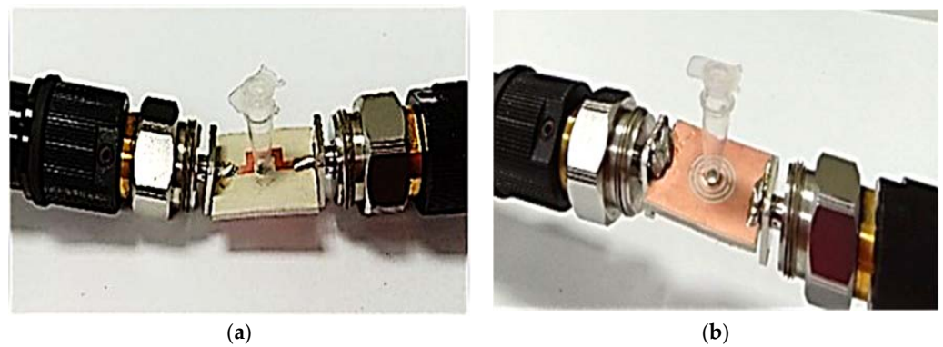
Figure 15. Position of PP tube loaded at the center of TR CSRR sensor; (a) Front and (b) side views.
