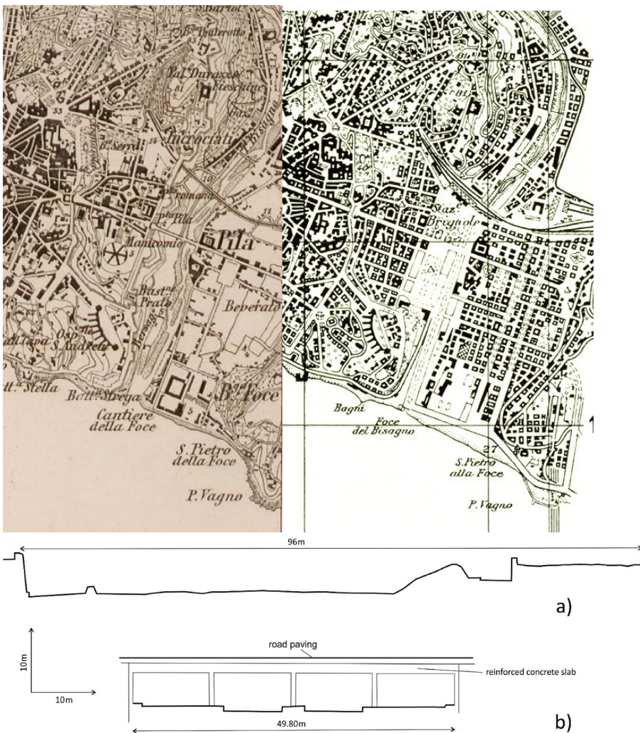
Figure 5. Historical map comparison (from Italian Military Geographical Institute maps, 1:25 000 scale, ed. 1878 and 1939) and corresponding stream cross-section at the mouth. (Modified from Inglese et al., 1909.)
