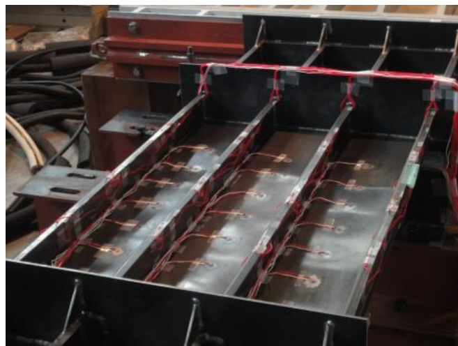
Figure 14: Collapse test of stiffened panel under cyclic compressive loading (Komoriyama et al., 2018b).
