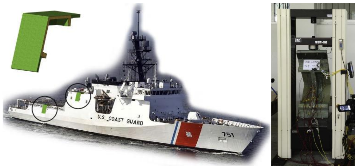
Figure 4: A sandwich composite L-Joint for ship structures under tension load. [Kai et al. 2020]
