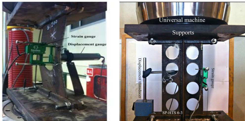
Figure 3: Experimental test setup, plate with one opening (left), stiffened plate with multiple openings (right)
