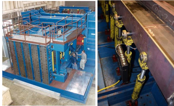
Figure A.4: (Left) Test fixture of the stiffened plate structure and (right) detailed view of the tie-downs and connection to the structure.
