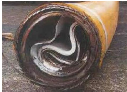
Figure 21: Collapse failure of a flexible riser caused by excessive hydrostatic pressure [Fernando, 2015].
