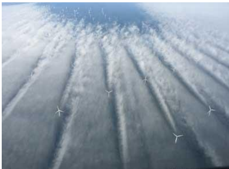
Figure 26: A photograph of the offshore wind farm at Horns Rev 2 Denmark was taken by helicopter pilot Gitte Lundorff. The photo of the fog over the sea dramatically pictured the offshore wind farm wake – which requires large offshore wind farms to be designed against both ultimate strength and fatigue resistance on a system level.
