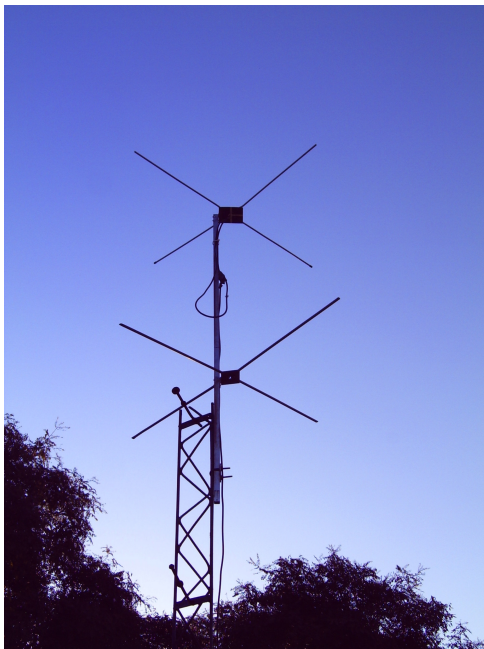
Figure 16 – Built Model of the Crossed Dipole Antenna.
