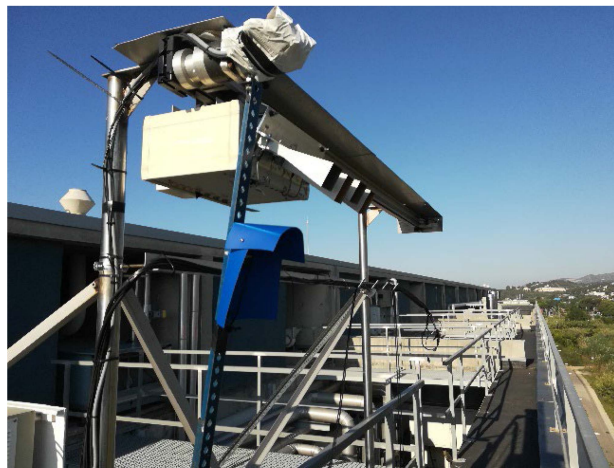
Fig. 2. GB-SAR instrument is deployed on the roof of the EEABB building, pointing to the experimental agricultural field.
