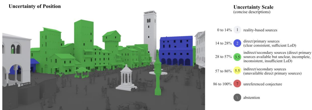
Figure 13. False-colour view of the uncertainty of the position of Piazza delle Erbe (the false-colour scale refers to Table 5).
