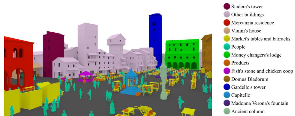
Figure 8. Subdivision of the 3D model of Piazza delle Erbe into families of analogous elements. At this stage, the colours of the scale of uncertainty had not been assigned yet, and random colours were assigned only to differentiate the various elements.
