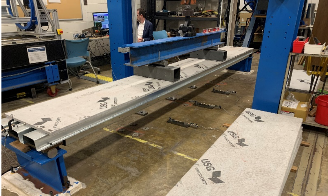
Figure 2. Four-point bending lab setup [1]
