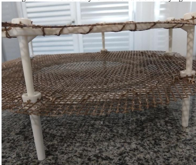
Figure 2 - Two-tier tray for microwave oven drying.
