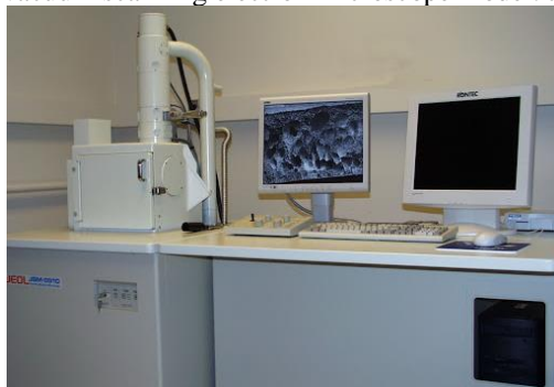
Figure 4. High vacuum scanning electron microscope model: JEOL JSM-5910
