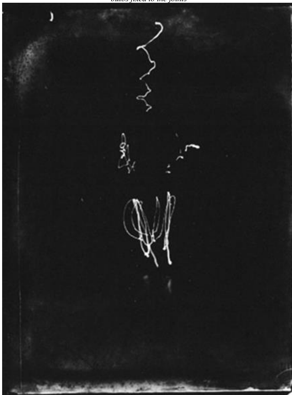
Figura 9. Marey, Etienne-Jules (1889) Pathological walk from in front, made visible by incandescent bulbs fixed to the joints
