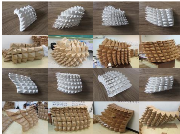
Figure 21: Comparison of the small size panels manufactured by addition and the panels constructed with cardboard in the 1: 1 scale.
