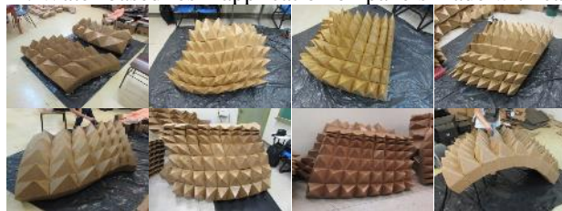
Figure 22: Water-based resin application on panels made with cardboard.
