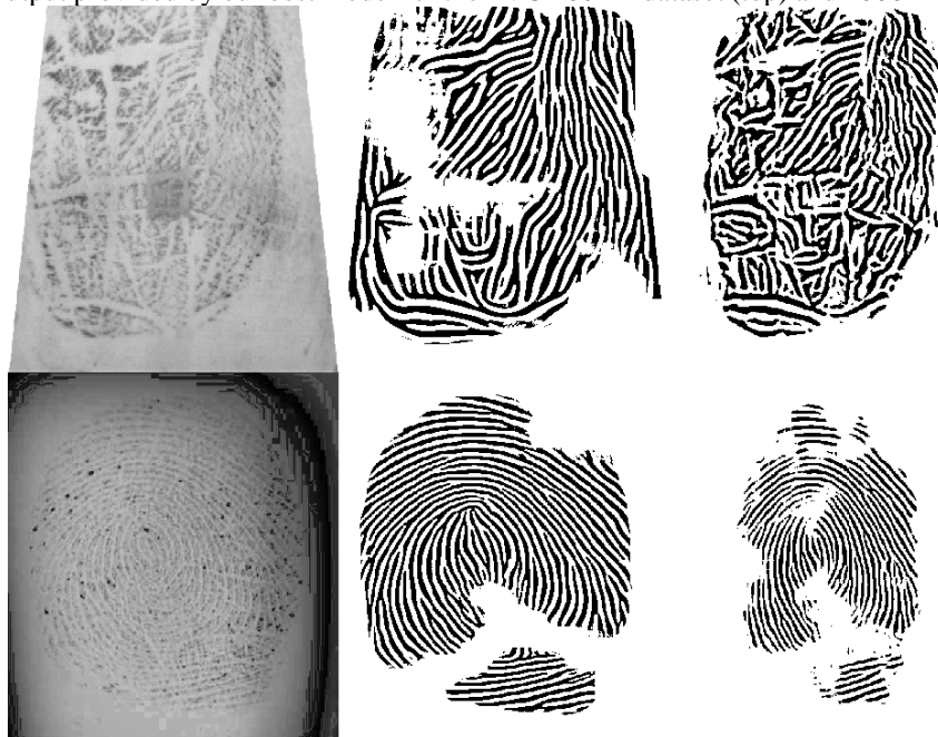
Figure.5 - From left to right: An example of an input image, the image used as ground truth, and the enhanced output provided by our best model for the FVC 2004-2 dataset (top) and 2006-2 dataset (bottom).
