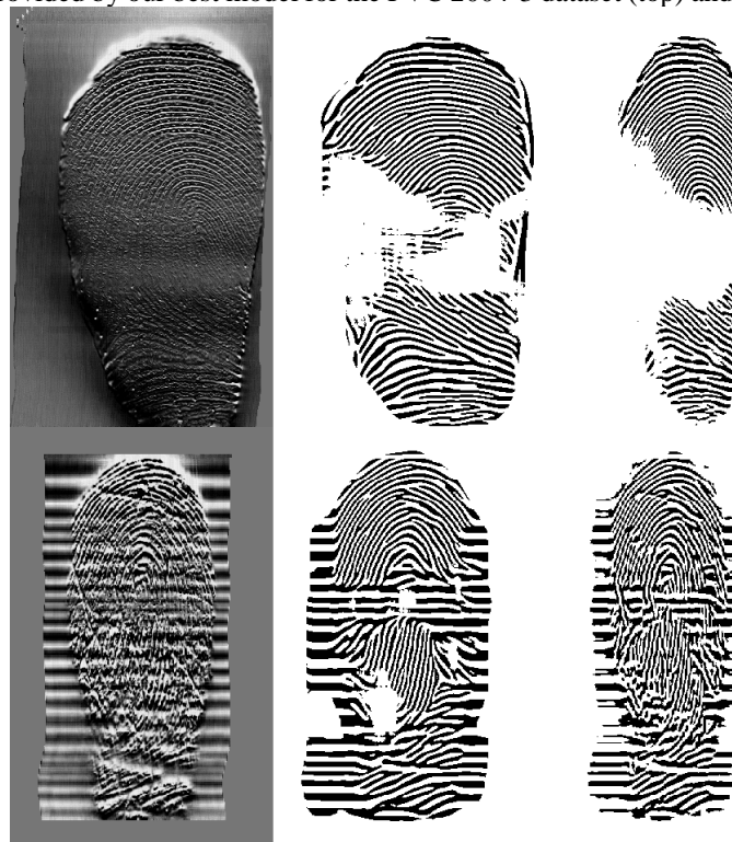
Figure.6 - From left to right: An example of an input image, the image used as ground truth, and the enhanced output provided by our best model for the FVC 2004-3 dataset (top) and 2006-3 dataset (bottom).
