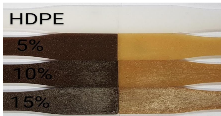
Figure 4 - Zoom of tensile strength specimen (left untreated fiber / right treated fiber)
