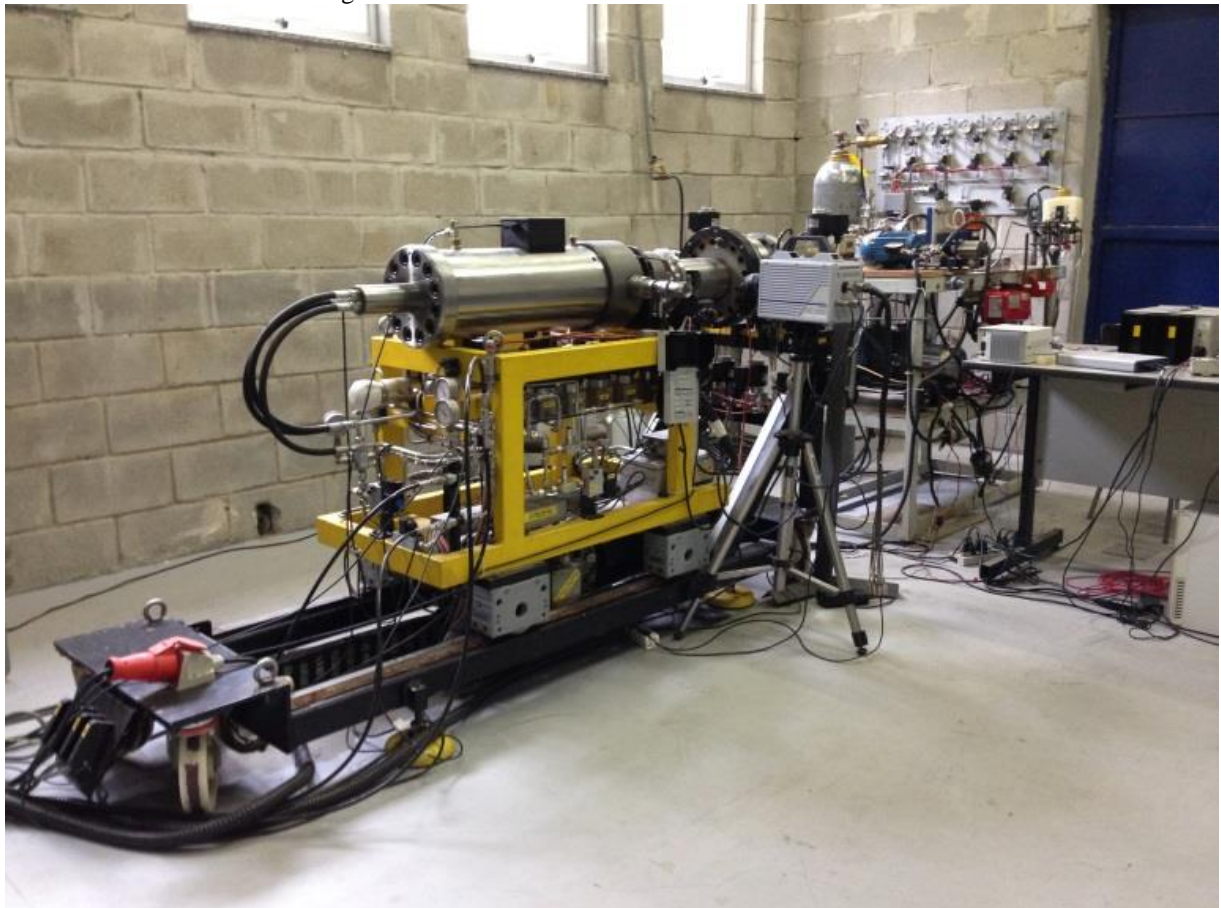
Figure 2. RCM installed on VEL at PUC – Rio.
