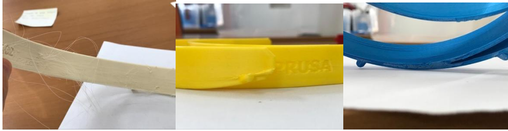
FIGURE 6 – Anomalies in the printing process. Source: LAB Archive (2020)
