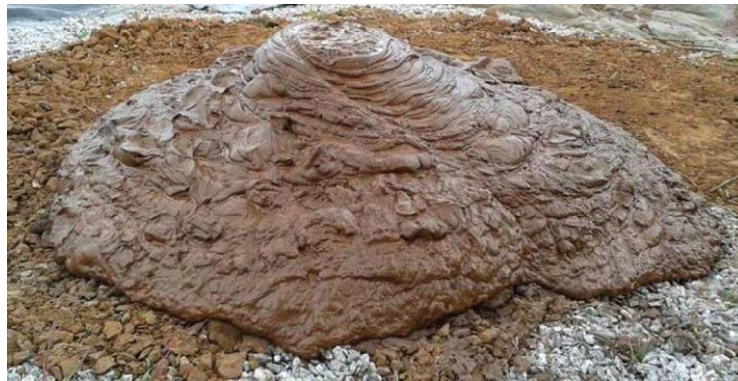
Figure 1 — Visual features of a sample of the iron ore tailing under paste consistence.
