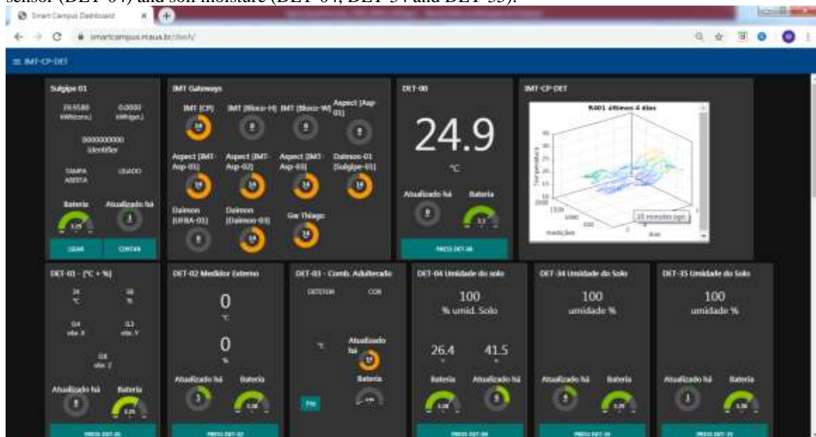
Fig.4. Smart Campus Mauá page showing the signals measured in the ambient temperature and humidity sensor (DET-04) and soil moisture (DET-04, DET-34 and DET-35).
