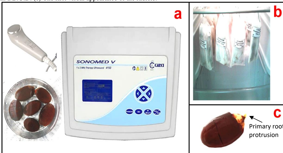
Figure 2: Seeds with ultrasound application: (a) Seeds submitted to an ultrasound device immersed in distilled water in a plastic cup. (b) Paper rolls containing 25 seeds distributed in a vertical position and kept in a B.O.D. (c) The first visual appearance of the radicle.
