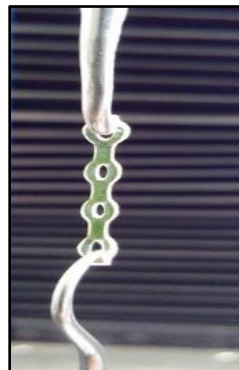
Figure 2. Hooks adapted to the universal testing machine to take readings.
