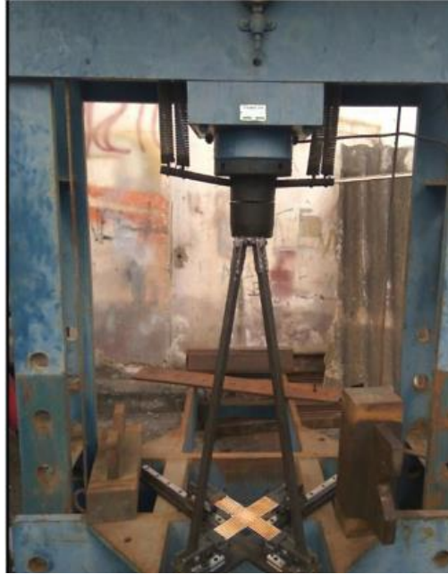
Figure 8: Biaxial tensile test setup for device stiffness testing.
