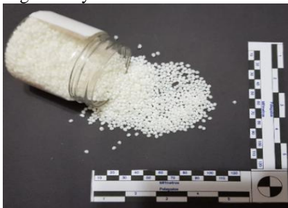
Fig. 3. Polymeric blend of PBAT/PLA
