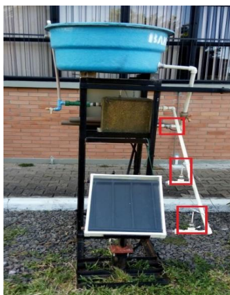
Figure 1: Alternative Solar Collector
