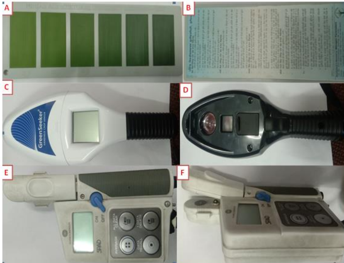
Fig. 6 Different gadgets advocated in the region for the site-specific nutrient management viz. Leaf colour chart A) Front and B) Rear side with guidelines in the local language; Green seeker C) Front and D) Rear side; Chlorophyll or SPAD meter E) Front side F) side view showing chamber where the leaf is to inserted (Source: Bhatt 2020 personal communication).
