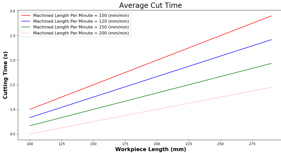
Figure 14: Cutting Time with Variations of the Workpiece Length.
