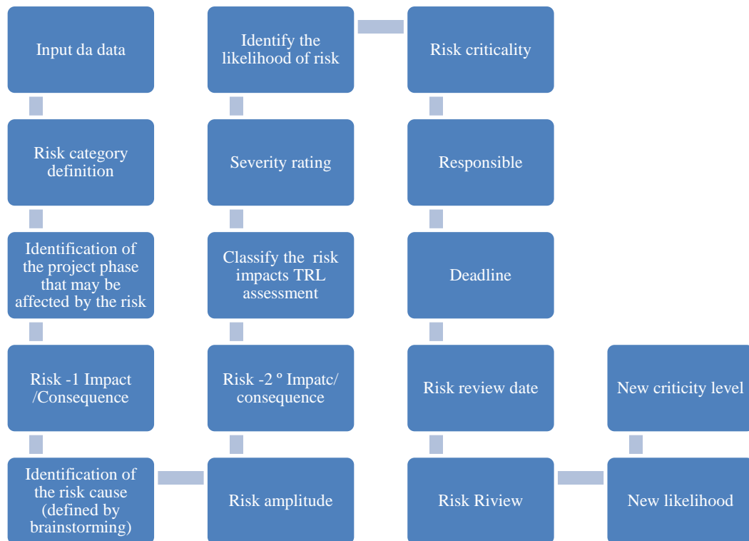
Figure 2. Risk record sheet – Risk Identification, Classification, Treatment and Monitoring. By the author
