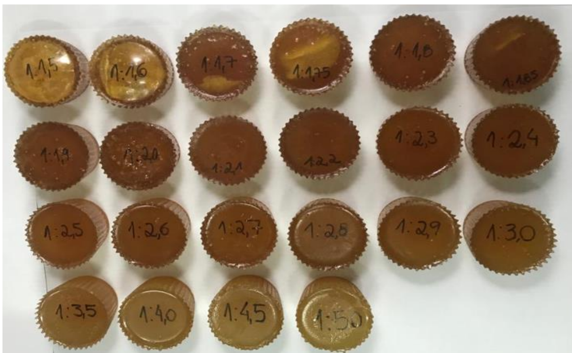
Figure 7 – Polyurethane resins with different ratios after curing time.
