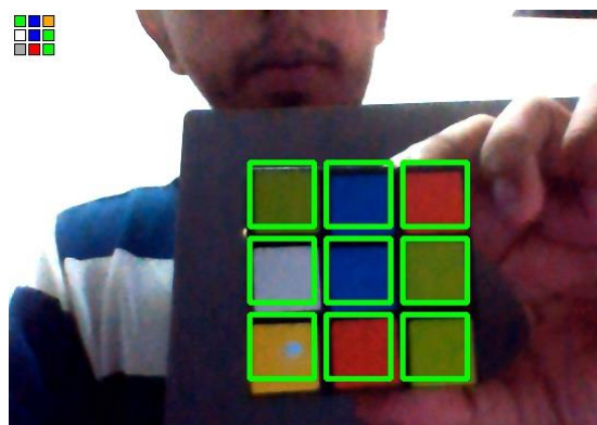
Figure 11: lower left block with reflection, reading was not possible, being shown the gray color in the upper left corner.
