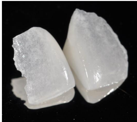
Figure 3: Ceramic fragments based on high translucency lithium disilicate (HT), in color A2.
